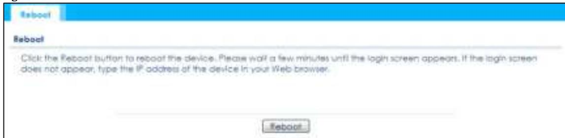
Click the **Reboot** button to restart the Zyxel Device. Wait a few minutes until the login screen appears. If the login screen does not appear, type the IP address of the Zyxel Device in your Web browser.
