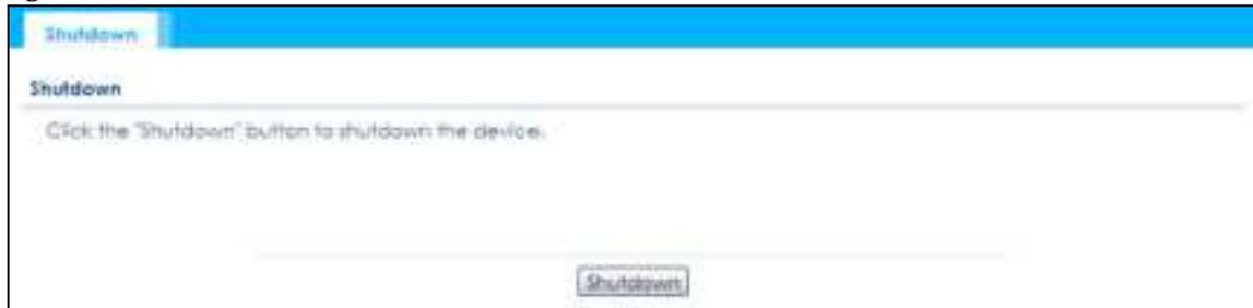
Click the **Shutdown** button to shut down the Zyxel Device. Wait for the Zyxel Device to shut down before you manually turn off or remove the power. It does not turn off the power.
