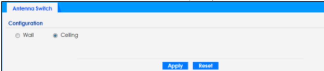
The screenshot shows the 'Antenna Switch' configuration page for a single AP. It features a blue header with 'Antenna Switch'. The 'Configuration' section has a checked checkbox for 'Enable Software Control'. Below this, there are two radio buttons: 'Wall' (unselected) and 'Ceiling' (selected). At the bottom, there are 'Apply' and 'Reset' buttons.
