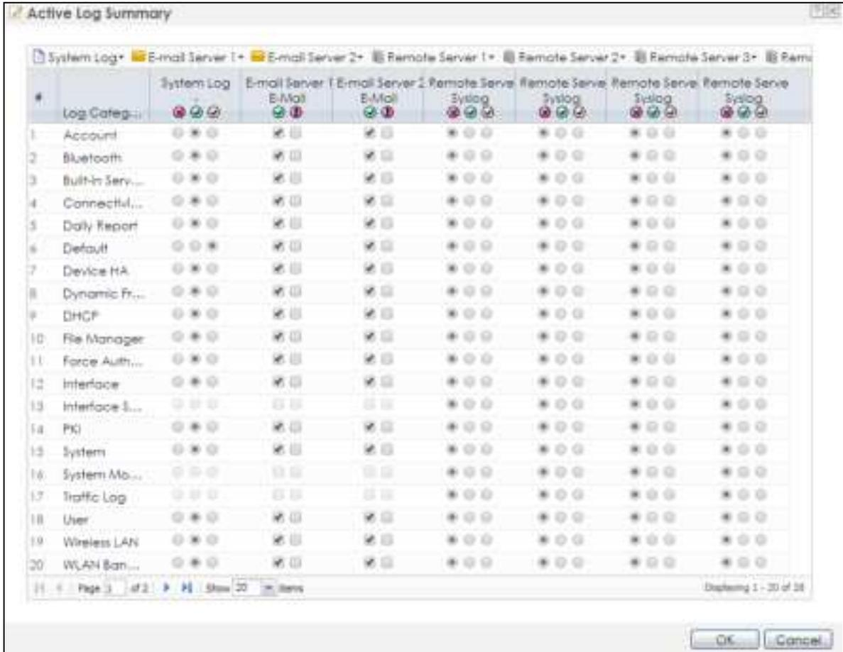
This screen provides a different view and a different way of indicating which messages are included in each log and each alert. (The **Default** category includes debugging messages generated by open source software.)
