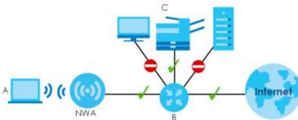
MAC addresses that are not listed in the layer-2 isolation table are blocked from communicating with the Zyxel Device's wireless clients except for broadcast packets. Layer-2 isolation does not check the traffic between wireless clients that are associated with the same AP. Intra-BSS traffic allows wireless clients associated with the same AP to communicate with each other.
