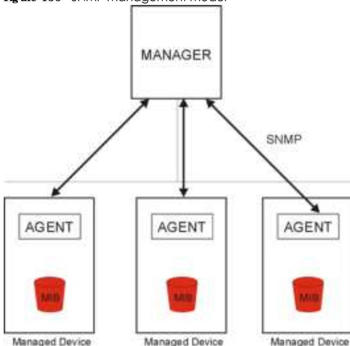
An SNMP managed network consists of two main types of component: agents and a manager.
