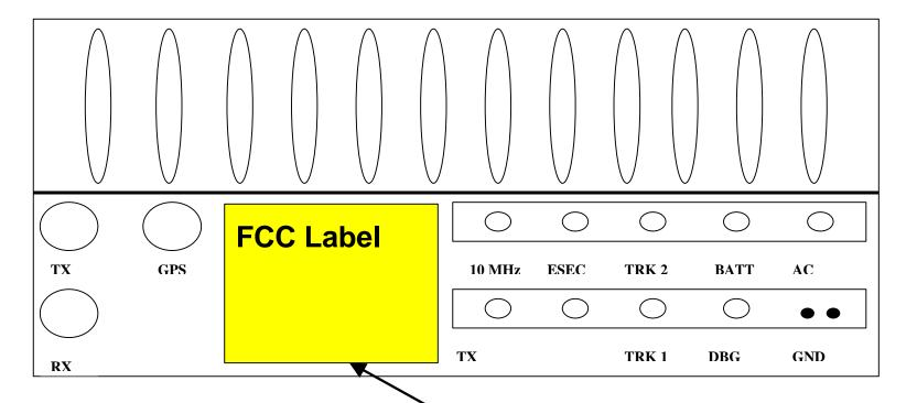
Label will be located on the bottom because PICO-BTS will be located on the pole or wall bottom side will be the most visible side. Furthermore, installer have to see the bottom side because most of the port is on the bottom side.
