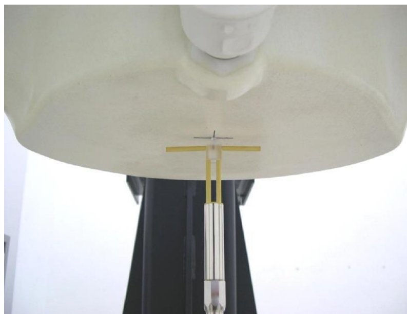
Picture 8.2 Photo of Dipole Setup
