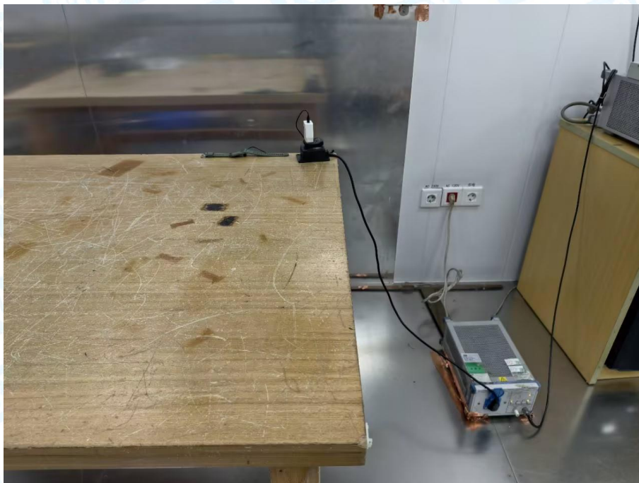
Photo of Setup for Conducted Emission
