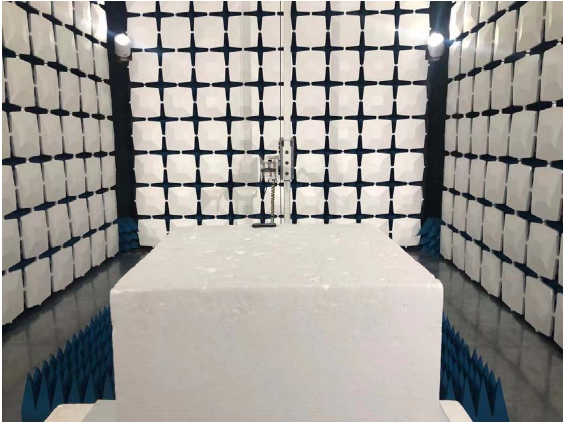
Above 1GHz for radiated emission test setup
