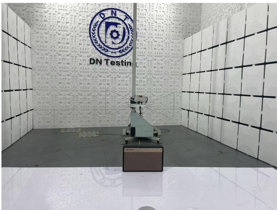
Radiated Emission Test View|(Below 1G)
