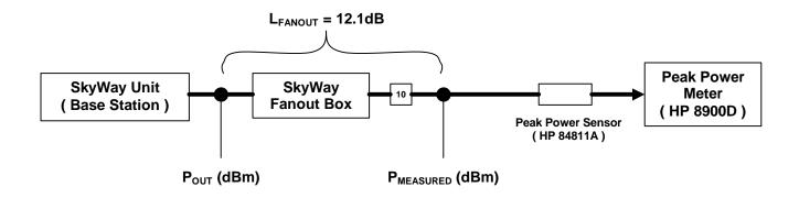
The power as referred to the Antenna port (P<sub>OUT</sub>) was calculated with the following equation:
