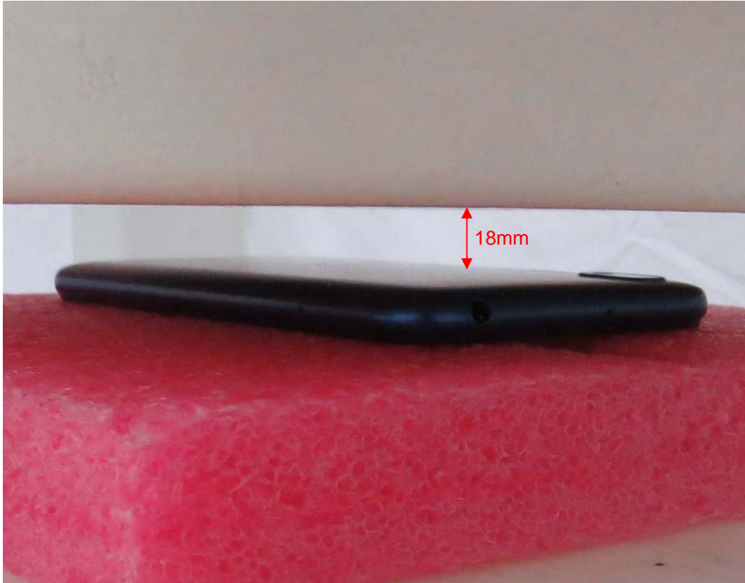
Picture 7: Back Side, the distance from handset to the bottom of the Phantom is 18mm
