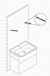
5.Drive a screw and an expansion plug into the hole.
