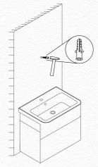
4.Drill the marks with an electric drill.
