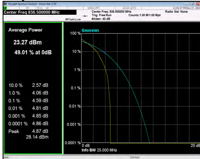
Band5 QPSK BW=1.4MHz Channel=20643 RB Size=1 Position=#0
