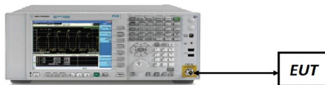
Figure 7-4. Test Instrument & Measurement Setup
