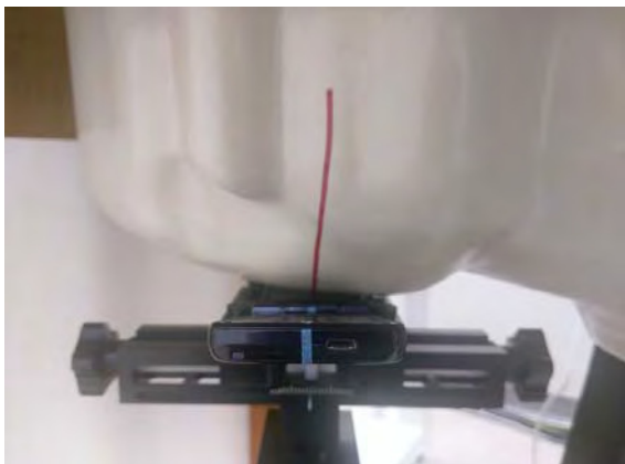
Fig.3 Right Head Section / Cheek-Touch Position
