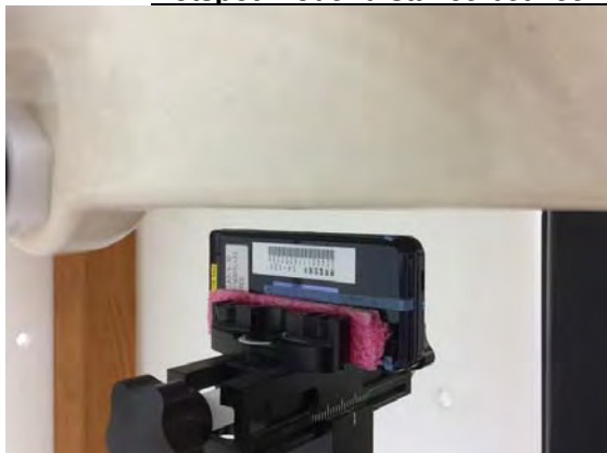
Fig.12 EUT Right side to flat phantom
