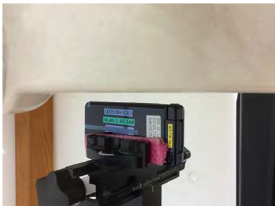
Fig.13 EUT Left side to flat phantom
