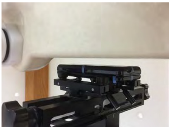
Fig.10 EUT Back side to flat phantom
