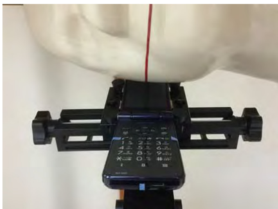
Fig.4 Right Head Section / Ear-Tilt Position(15°)
