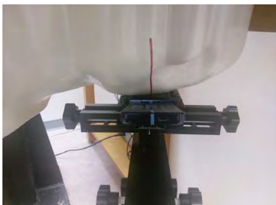
Fig.5 Left Head Section / Cheek-Touch Position
