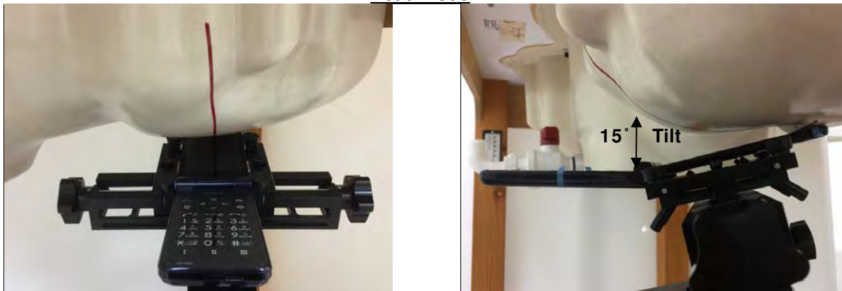
Fig.6 Left Head Section / Ear-Tilt Position(15°)
