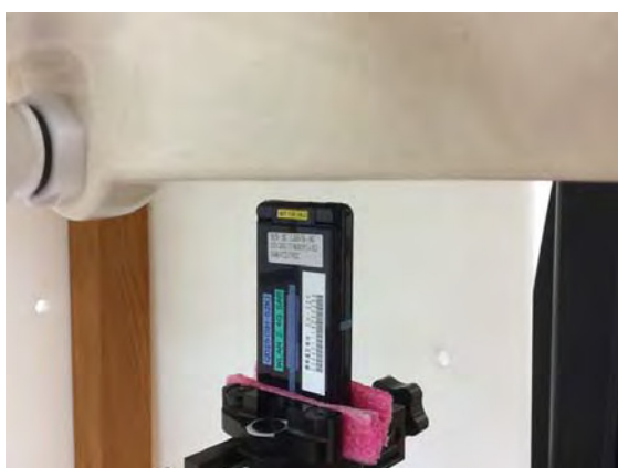
Fig.11 EUT Top side to flat phantom
