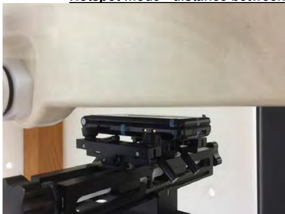
Fig.9 EUT Front side to flat phantom
