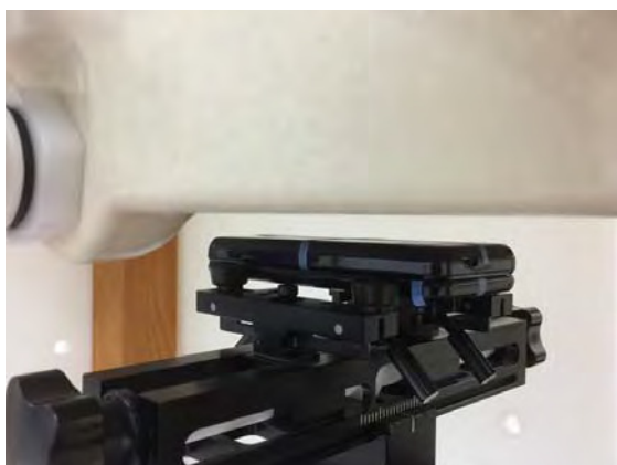
Fig.8 EUT Back side to flat phantom
