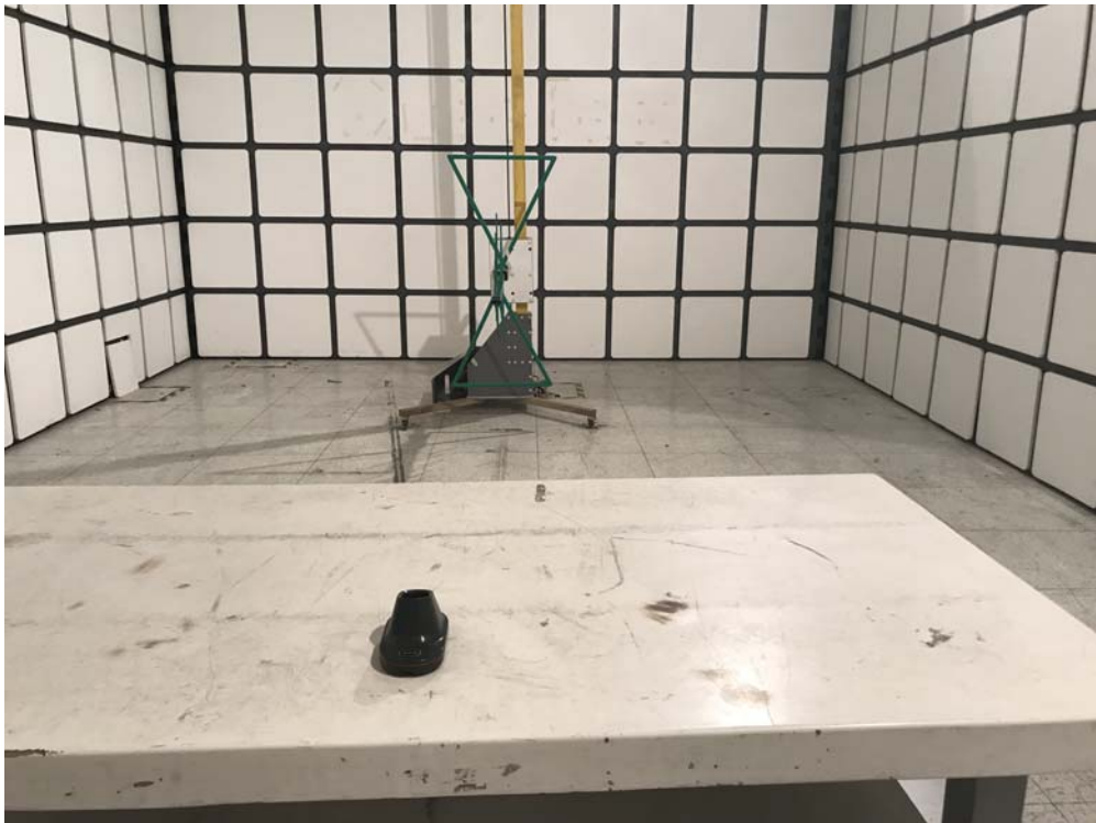
Description: Radiated Emission Test Setup for 1~18GHz
