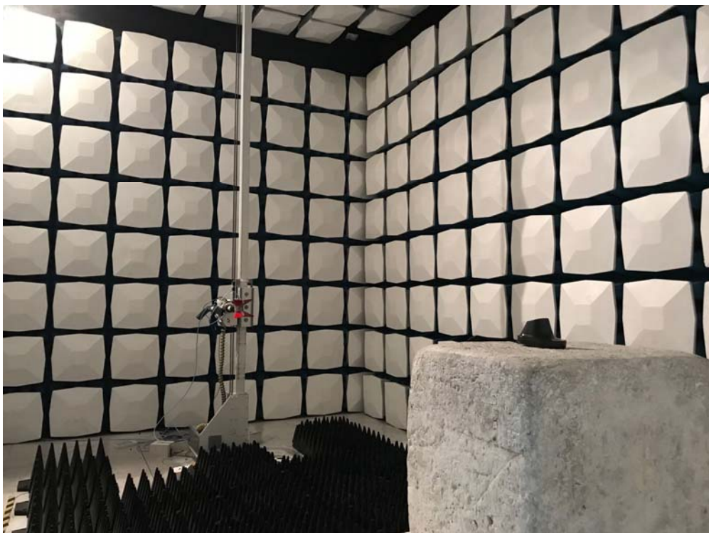
Description: Radiated Emission Test Setup for 1~18GHz
