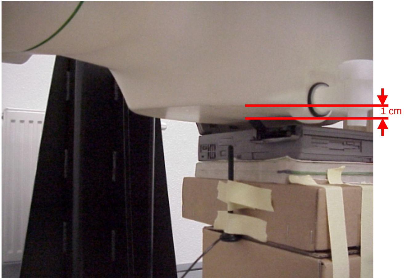
Photo 3: Position up side on the flat phantom (Body SAR measurement)
