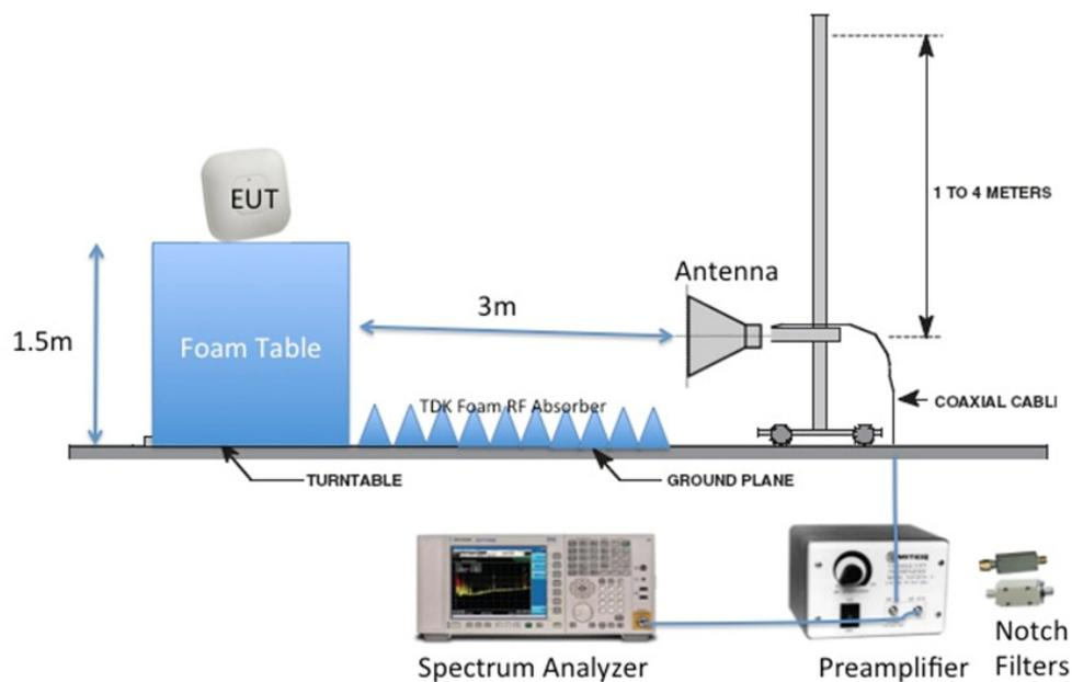
**Note:** The radiated spurious emissions test setup referenced to KDB789033 D02, v02r01, Section II (G)(3)(b)(i)), the EUT antenna ports were terminated with 50Ω loads.
