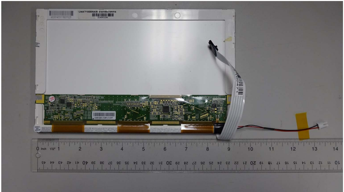
LCD Panel (Rear View)
