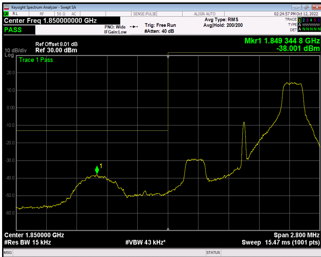
Band2 QPSK BW=1.4MHz Channel=18607 RB Size=6 Position=#0
