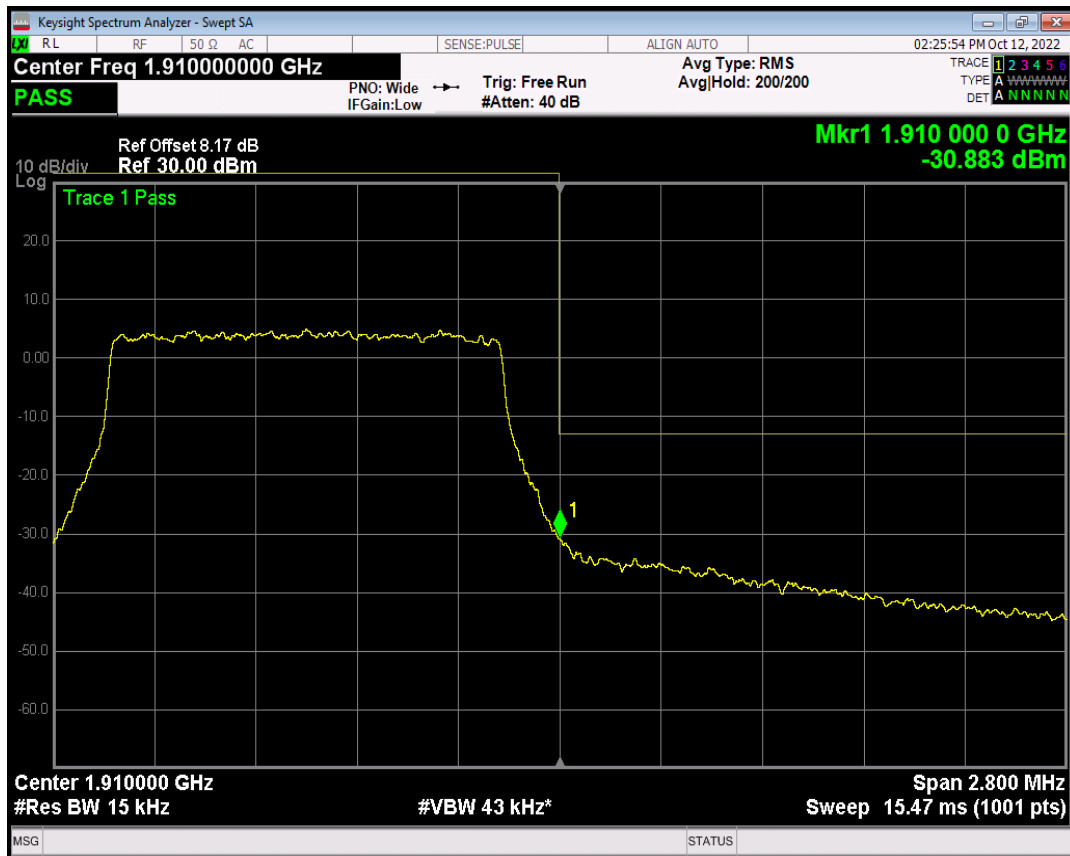
Band2 QPSK BW=3MHz Channel=18615 RB Size=1 Position=#0
