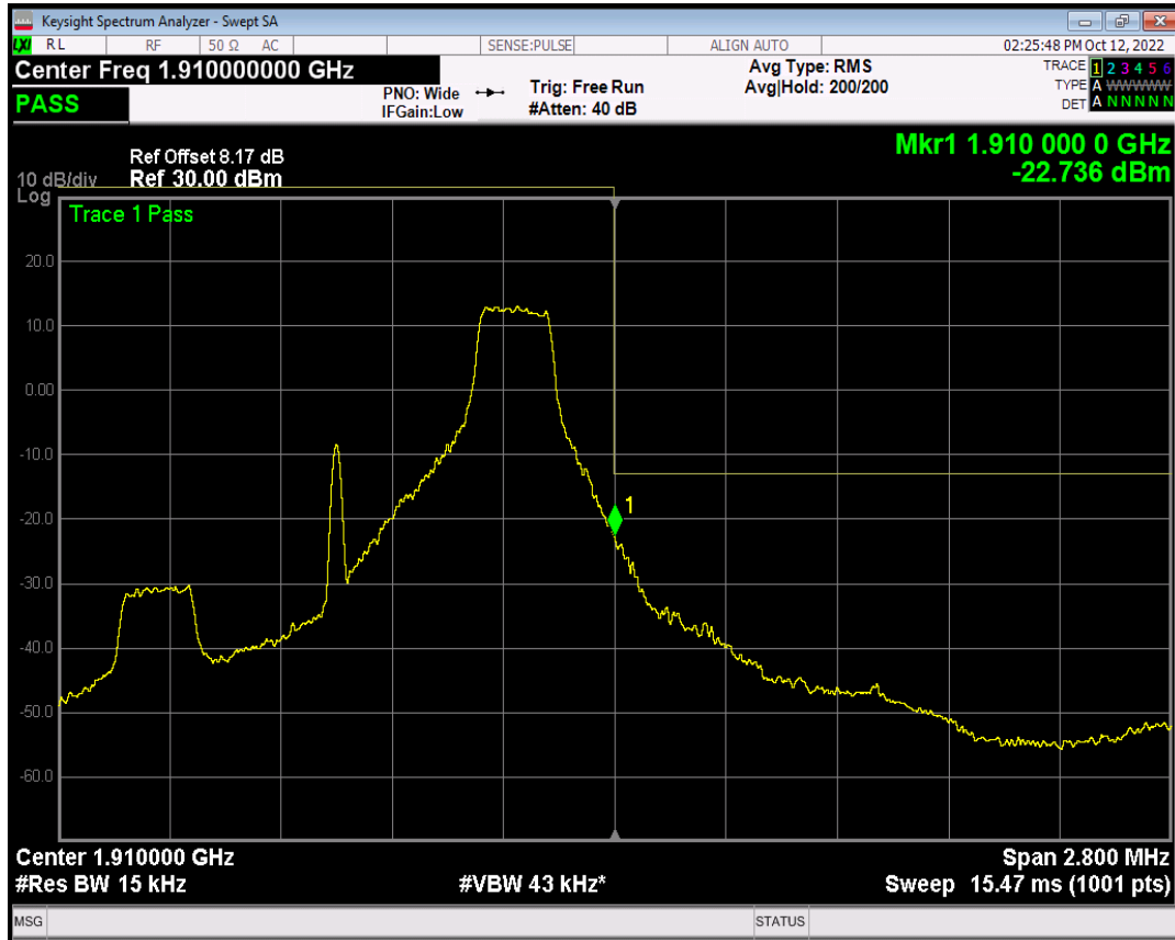
Band2 QAM16 BW=1.4MHz Channel=19193 RB Size=6 Position=#0
