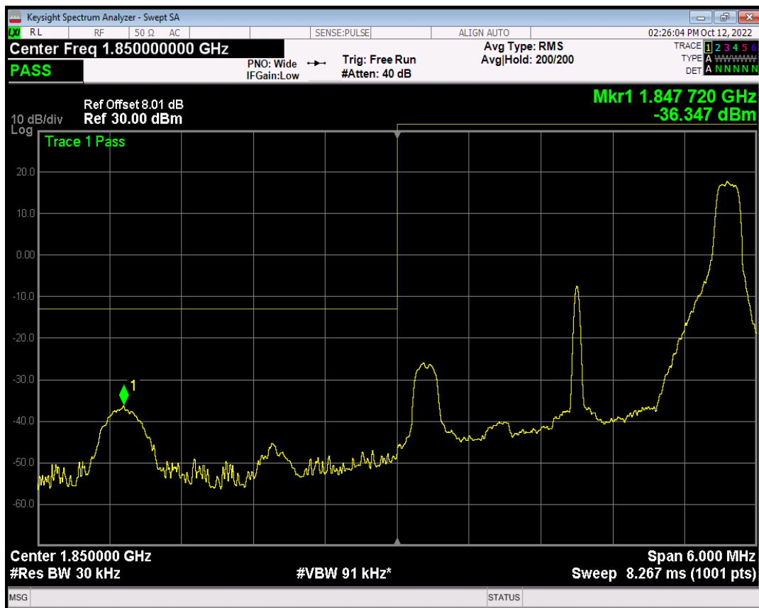
Band2 QPSK BW=3MHz Channel=18615 RB Size=15 Position=#0
