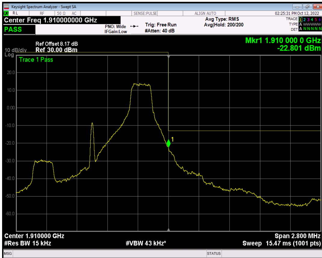
Band2 QPSK BW=1.4MHz Channel=19193 RB Size=6 Position=#0
