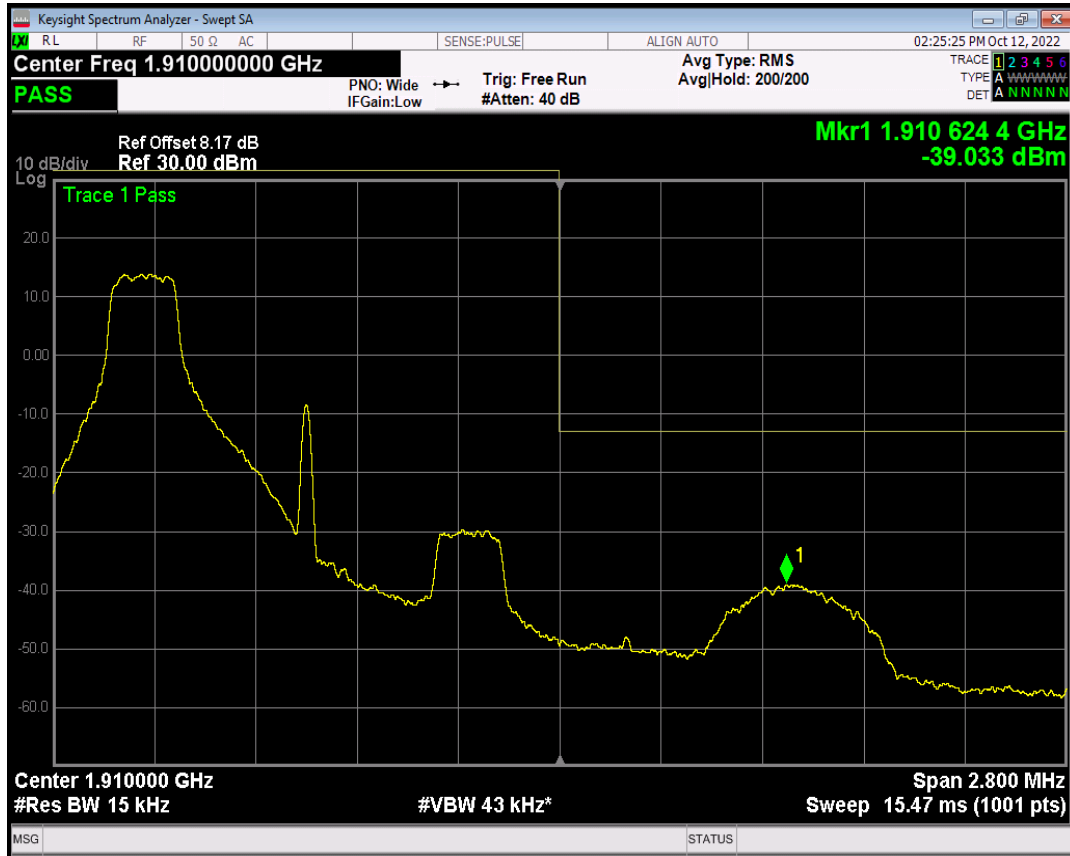
Band2 QPSK BW=1.4MHz Channel=19193 RB Size=1 Position=#Max
