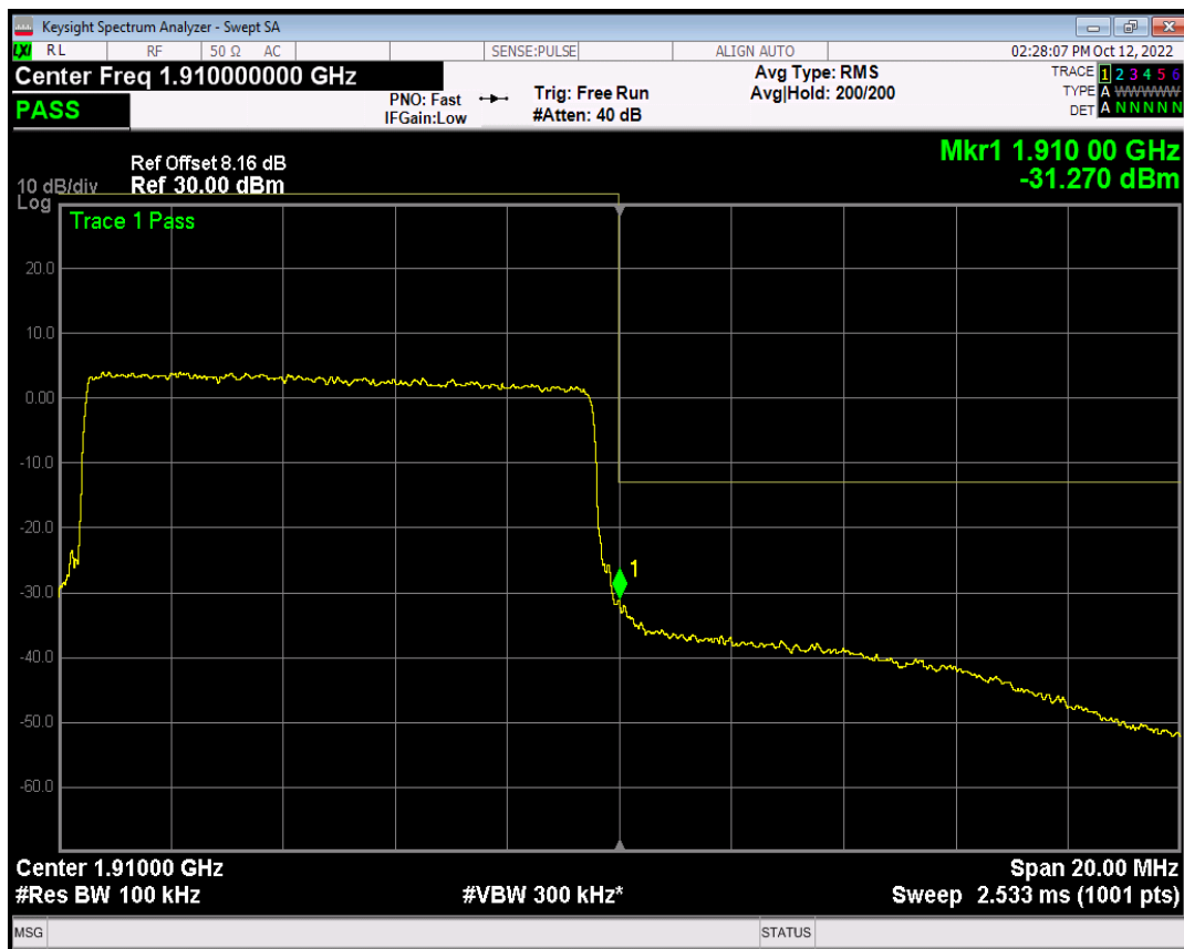
Band2 QPSK BW=15MHz Channel=18675 RB Size=1 Position=#0
