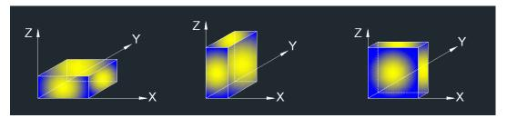
Note 1: The manufacturer has recommended that the EUT only be used in the desktop (horizontal)orientation; therefore, all radiated testing was performed in desktop orientation(X).
