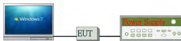
Fig. 2-2 Conducted (Antenna Port) Configuration Emission
