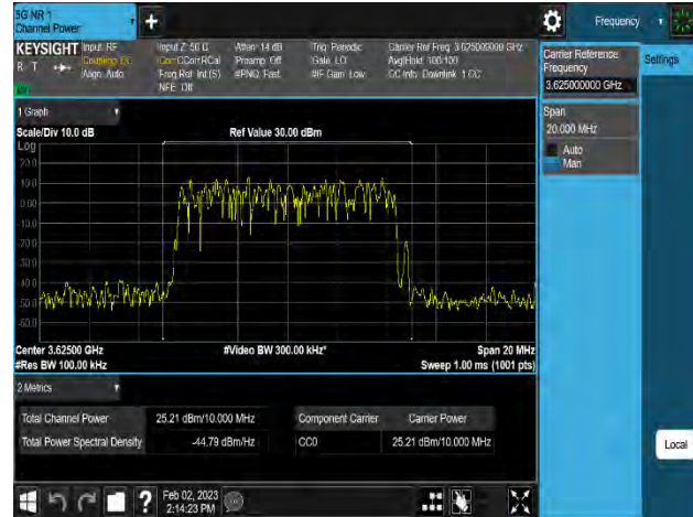
Plot 8-223. Equivalent Isotropic Radiated Power Plot (n48_1C_10M_QPSK - Mid Channel_8T, Port 8)
