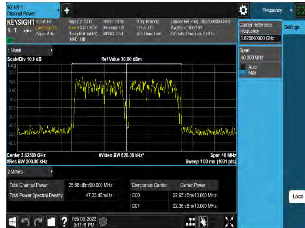
Plot 8-231. Equivalent Isotropic Radiated Power Plot (n48_2C_10M+10M_16QAM - Mid Channel_8T, Port 8)
