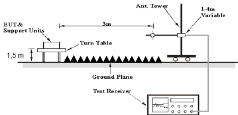
The radiated emission below 1GHz tests were performed in the 10 meters chamber, above 1GHz tests were performed in the 3 meters chamber A, using the setup accordance with the ANSI C63.10-2013. The specification used was the FCC 15.209, and FCC 15.247 limits.
