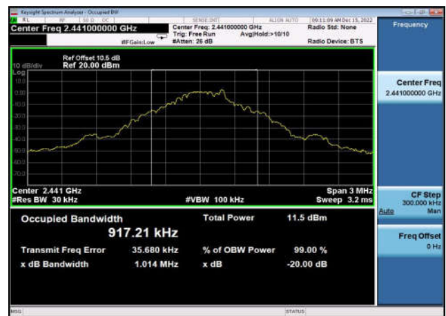
20dB Bandwidth: DQPSK,2402MHz,2DH5
