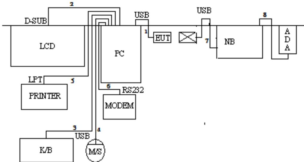
1. The USB cable is connected from the PC to the EUT.
