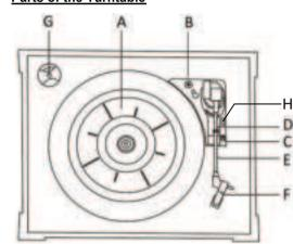
B. Safety Screw (for transport) Before using the unit, turn the screw clockwise using a coin or
