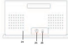
24. FM wire antenna While tuned to a station in FM mode, extend the wire and reposition to adjust for best reception. 25. LINE OUT lacks For amplifier device with RCA auxiliary input sockets, insert the white and red plugs on the RCA cable into the unit. Insert the opposite end into the amplifier device. Be sure to connect the white plug to the white jack and the red plug to the red jack. 26. Power Adaptor Connect the Power adaptor into a wall outlet. It is strongly recommended that this product
