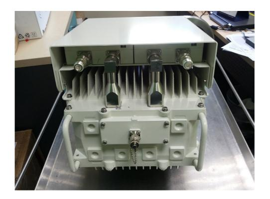
Photograph No.2 "AirHarmony 4000 2.5 GHz (B41)" base station front side view
