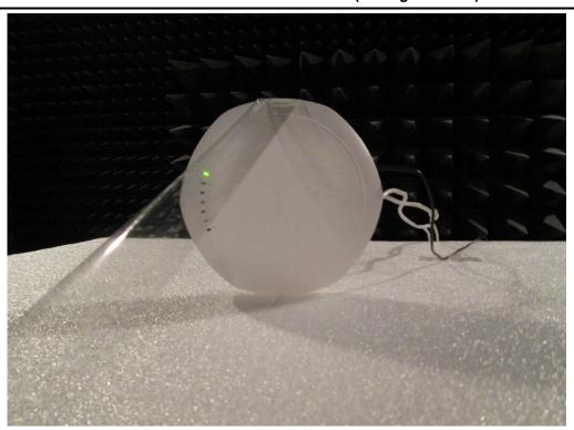
Radiated Emission Above 1GHz Test (Wall mounted)
