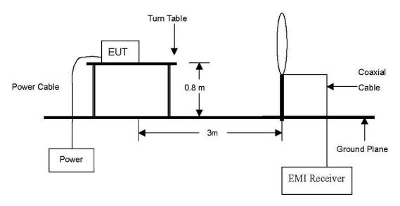
The diagram below shows the test setup that is utilized to make the measurements for emission from 30  $\,\text{Mz}$  to 1  $\,\text{GHz}$  emissions.
