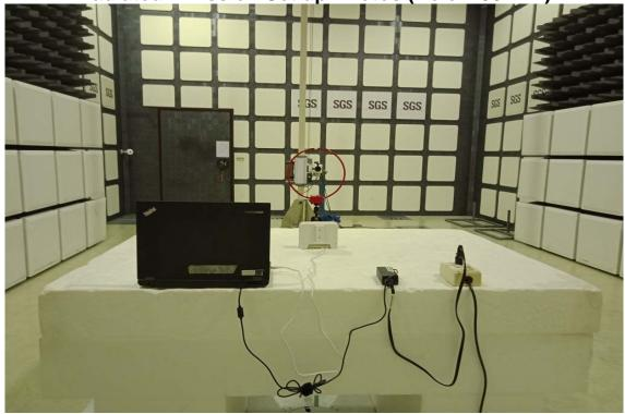
Radiated Emission Set up Photos (Below 1GHz)
