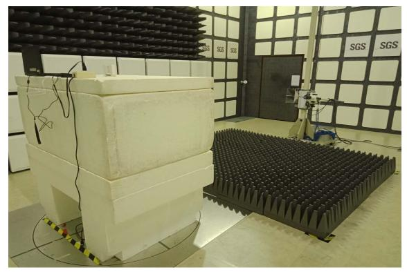
Radiated Emission Set up Photos (Front View)
