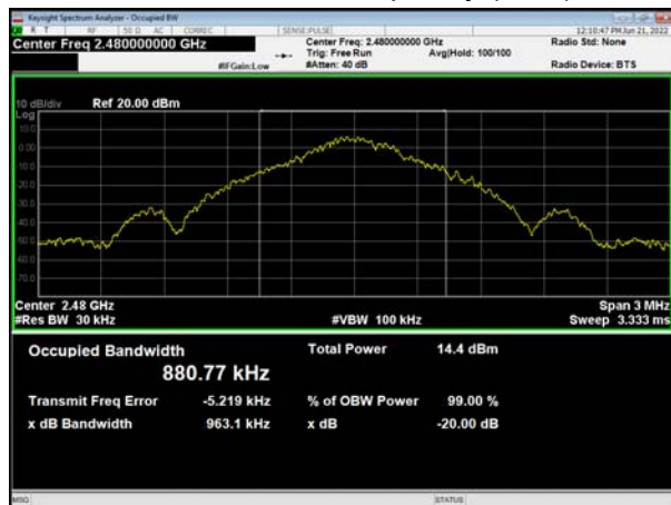
BT DH5 CH78, Carrier frequency (MHz): 2480
