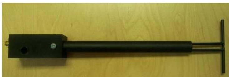
Figure 1 – MVG COMOSAR Validation Dipole
