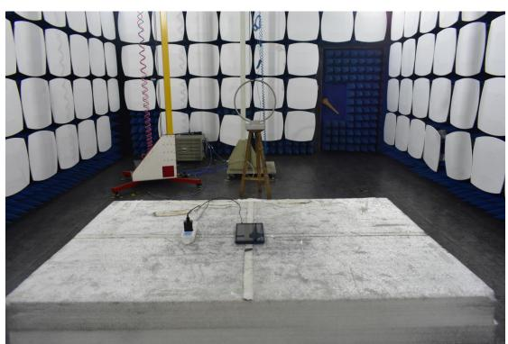
3. Radiated emission (9KHz-30MHz)
