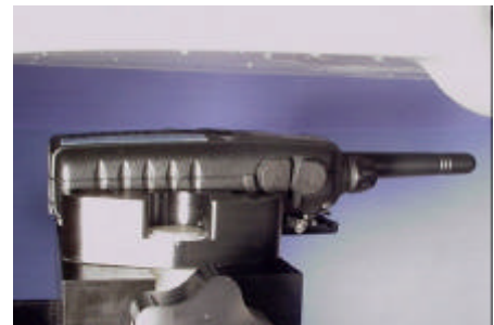
Face-held SAR Test Setup 2.5cm Separation Distance
