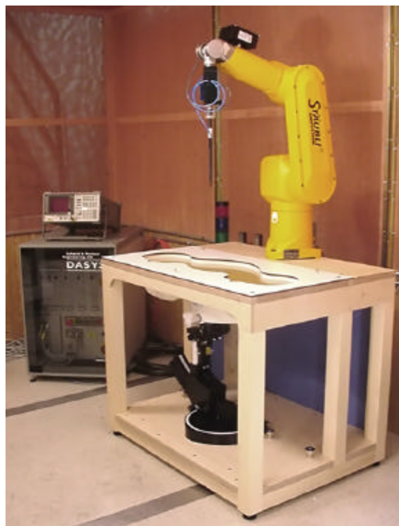
DASY3 SAR Measurement System with SAM phantom
