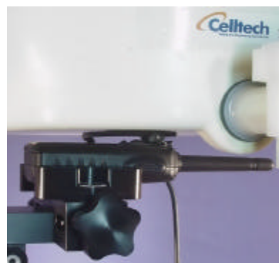
Body-worn SAR Test Setup with 1.0cm Belt-Clip & Speaker-Mic
