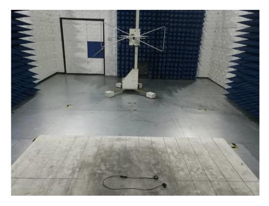
RADIATED EMISSION TEST SETUP ABOVE 1GHZ
