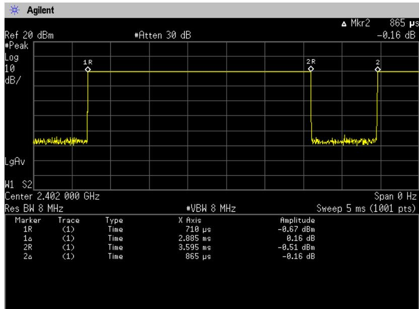
$$\text{Duty Cycle} = T_{\text{on}} / (T_{\text{on}} + T_{\text{off}}) = 2885[\mu\text{s}] / (2885[\mu\text{s}] + 865[\mu\text{s}]) = 76.9[\%]$$
