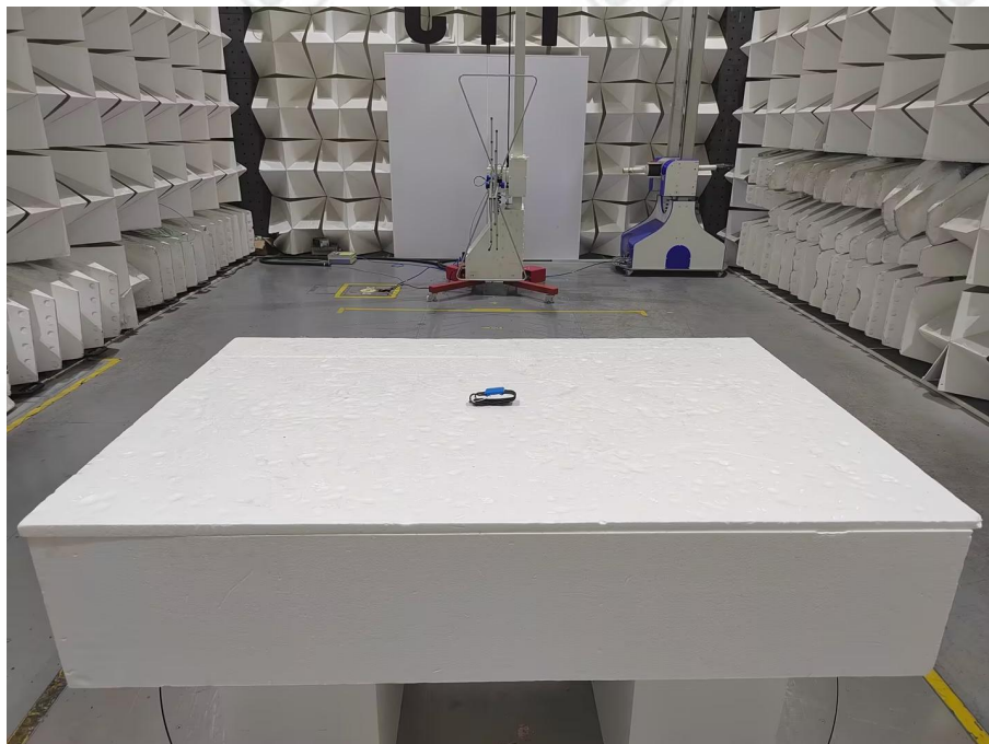
Radiated emission Test Setup-1 (30MHz~1GHz)
