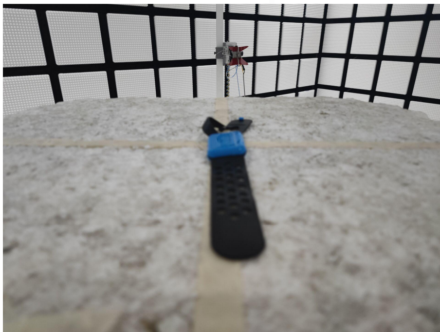
Radiated spurious emission Test Setup-3(Above 1GHz)
