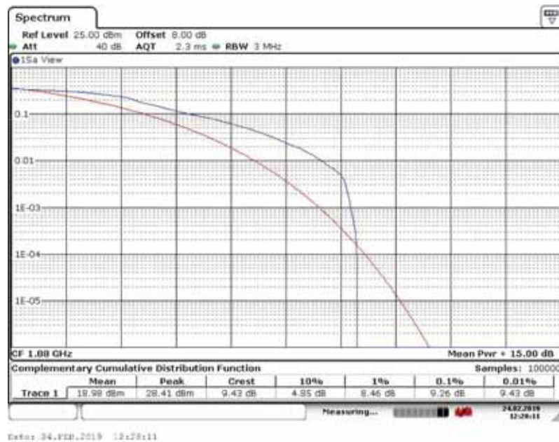
Peak-Average Ratio Plot(20MHz BW,16QAM,Band 2-mid Channel)
