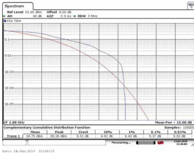
Peak-Average Ratio Plot(3MHz BW,16QAM,Band 2-mid Channel)
