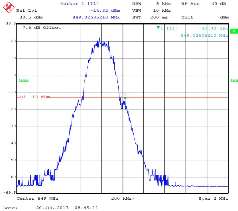
**Cellular Band, Left Band Edge for WCDMA (BPSK) Mode**
