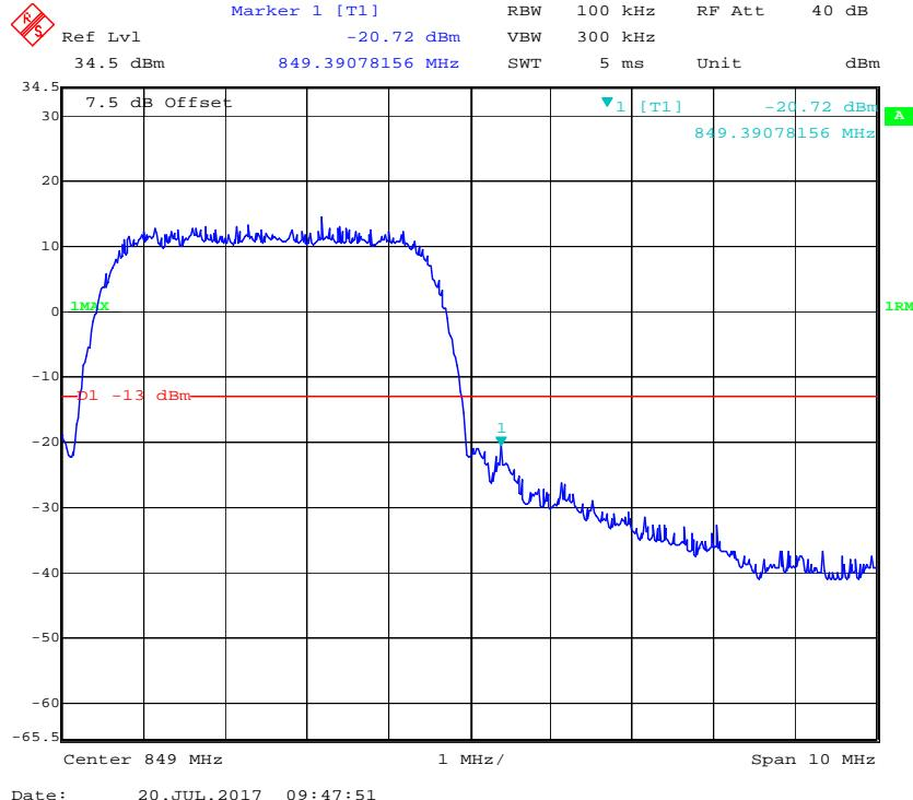
**PCS Band, Left Band Edge for GSM (GMSK) Mode**
