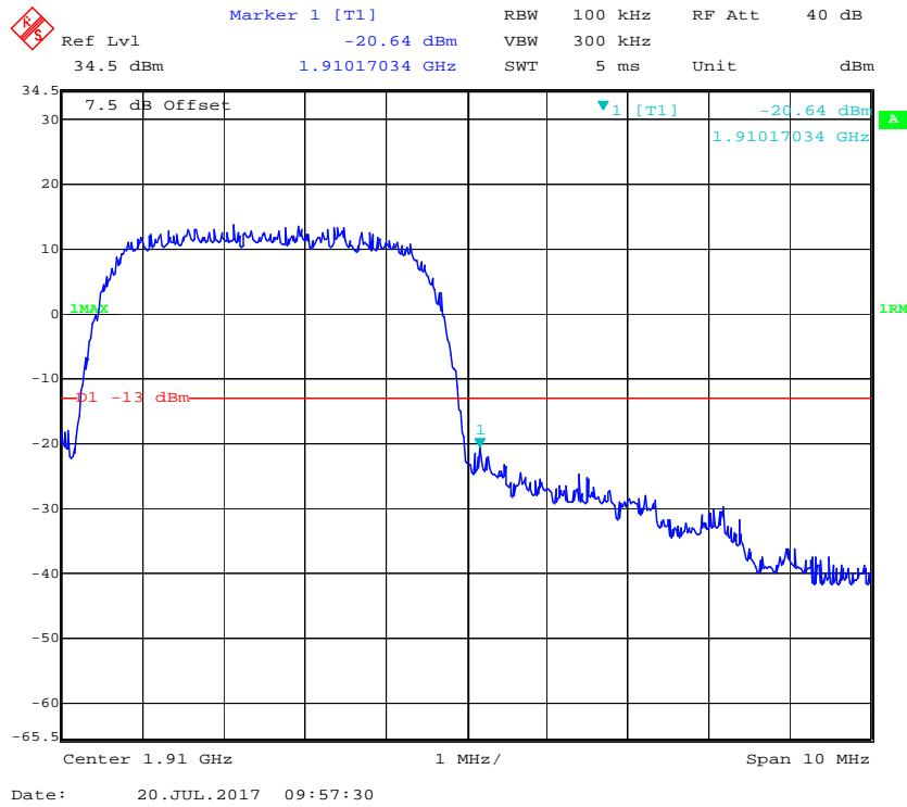
**PCS Band, Left Band Edge for HSUPA (BPSK) Mode**
