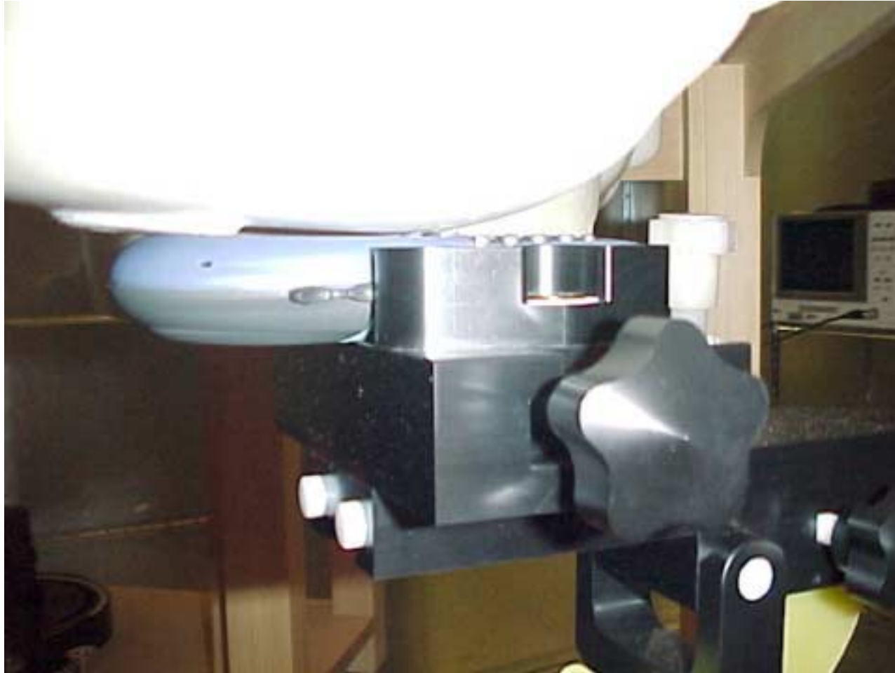
Position of device against head phantom using the “cheek” position
