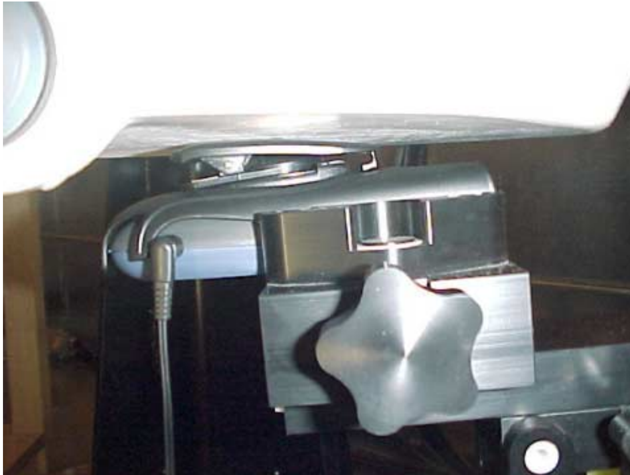
Position of device against flat phantom using carry accessory SXX 109 4705 with hands free accessory RLF 501 25/03
