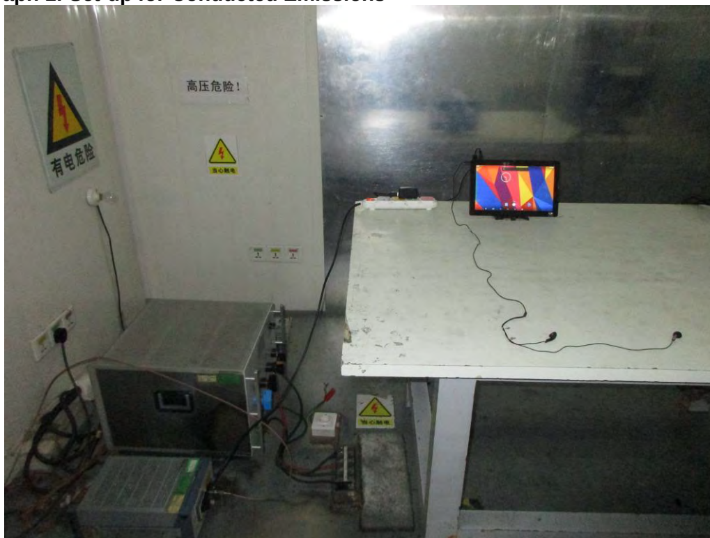
Photograph 2: Set-up for Spurious Emissions for below 30MHz
