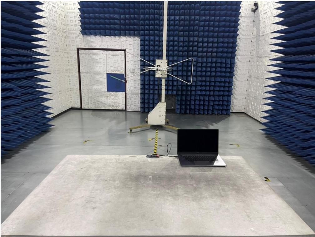
RADIATED EMISSION TEST SETUP ABOVE 1GHZ-NORA-B100 OF ANT 1
