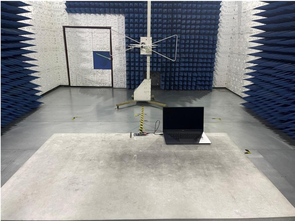
RADIATED EMISSION TEST SETUP BELOW 1GHZ-NORA-B101 OF ANT 2
