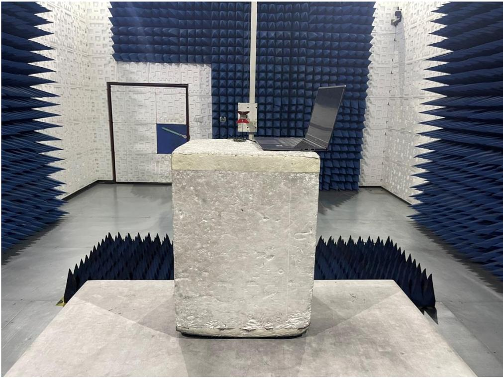
RADIATED EMISSION TEST SETUP ABOVE 1GHZ-NORA-B101 OF ANT 1
