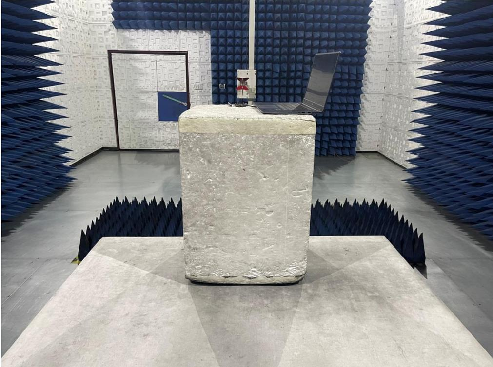
RADIATED EMISSION TEST SETUP ABOVE 1GHZ-NORA-B101 OF ANT 2
