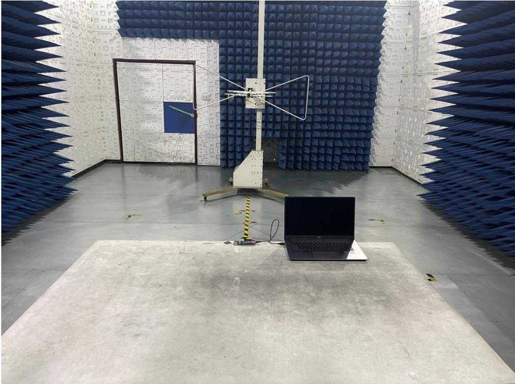
RADIATED EMISSION TEST SETUP BELOW 1GHZ-NORA-B106
