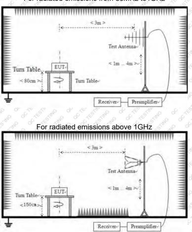
For radiated emissions from 30MHz to1GHz
