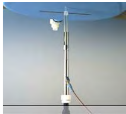
Photograph of the dipole Antenna
