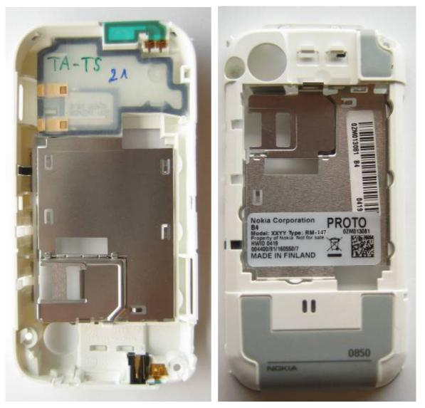
1.4 D-Cover with GSM-Antenna, BT-Antenna and Speaker
