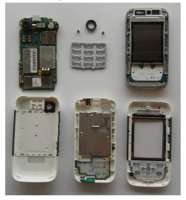
1.2 Phone after disassembling PWB and A-Cover
