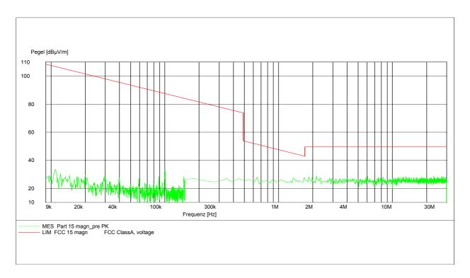
Settings: For peak measurement For QP measurement
