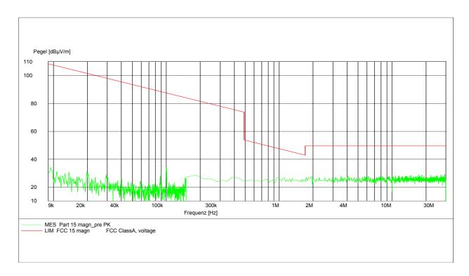
Settings: For peak measurement 100 kHz RBW/VBW For QP measurement 200 Hz for 9 kHz to 150 kHz
