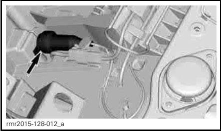
DC56 - REAR CUSTOMER ACCESSORY CIRCUIT - UNDER PASSENGER SEAT
