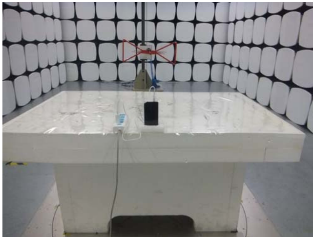
Radiated Spurious Emissions Test Setup Below 1GHz
