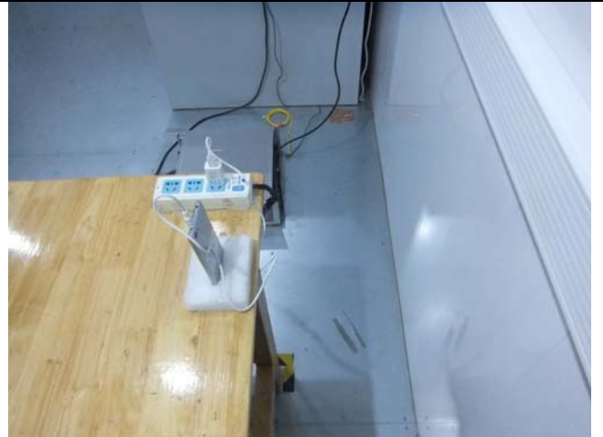
Conducted Emissions Test Setup Side View
