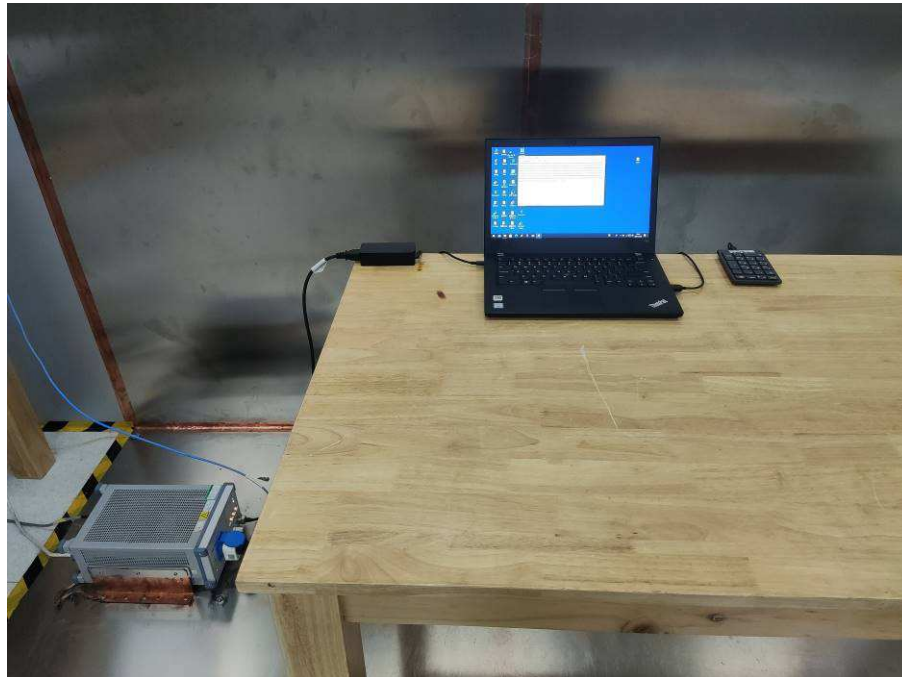
Photograph 3: Set-up for Conducted Emission on AC Mains
