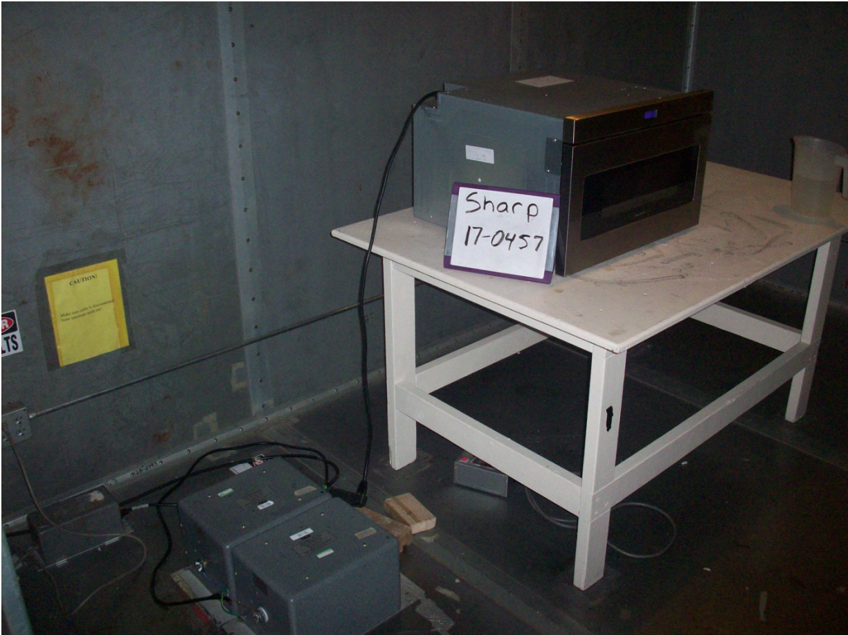
Figure 6. Conducted Emissions Measurement Photo
