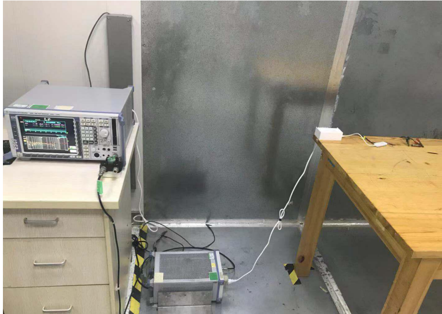
Radiated Spurious Emissions Test Frequency From 30MHz-1000MHz
