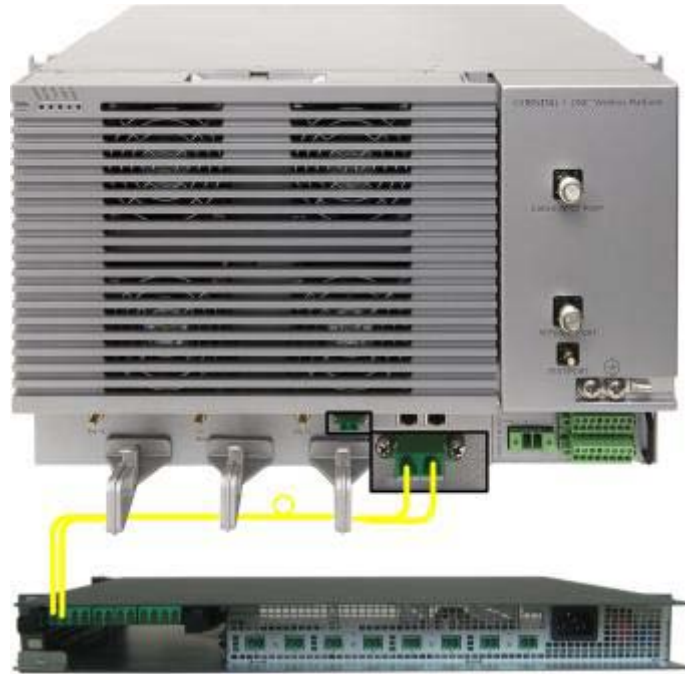
Figure 4-6 Fiber Connections toward ICU
